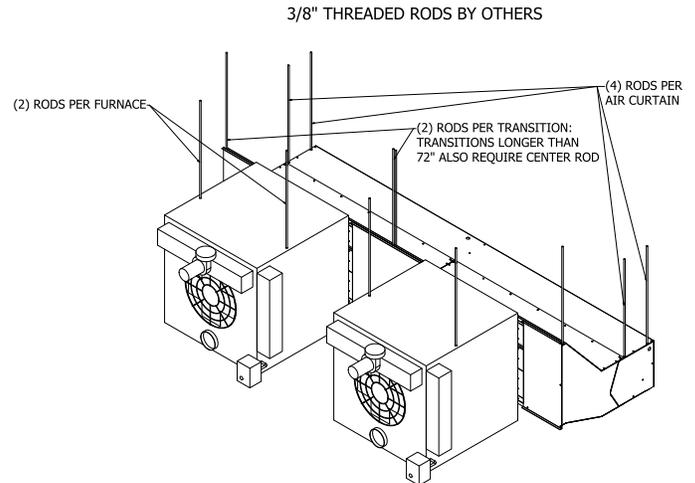
FIG. 5 (Indirect Gas Fired Heated HV2 Unit)
