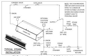
FIG. 4 (Steam Heated STD2 Unit)
